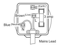
The wire coloured BLUE must be connected to the terminal marked N or coloured BLACK. The wire coloured BROWN must be connected to the terminal marked L or coloured RED.
